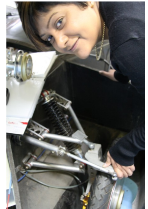
Shainaz measures suspension components for design checks
