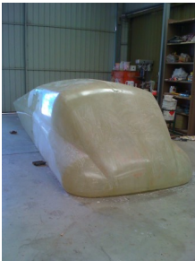
First test fibreglass shell
